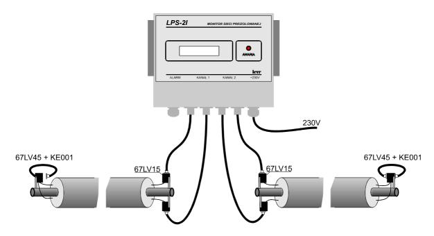
All connections should be made using coaxial cables of the 67LVxx type and 67LV15 and 67LV45 junction boxes. As a last resort, the ends of the copper wires of the alarm system can be directly shorted together.
