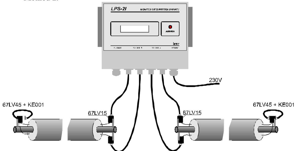
All the connections should be made with concentric cables type: 67LVxx and junction boxes 67LV15 and 67LV45. Under extreme circumstances the ends of the copper wires of the sensor loop can be connected directly.
